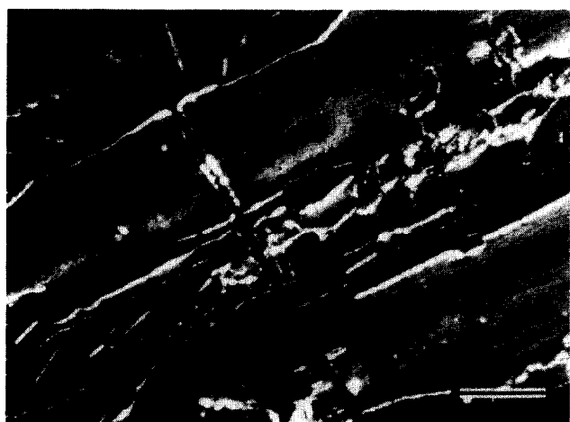
Figure 1 Optical micrograph of a highly oriented and birefringent POK layer taken after selective dissolution of the hydroquinone substrate crystals. Crossed Nicols; scale bar = 50 \mu\text{m}
